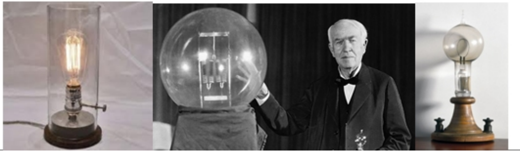
9. ábra Figure9 Edison's lamp had a single loop of carbon which glowed when a current flowed through it 9
